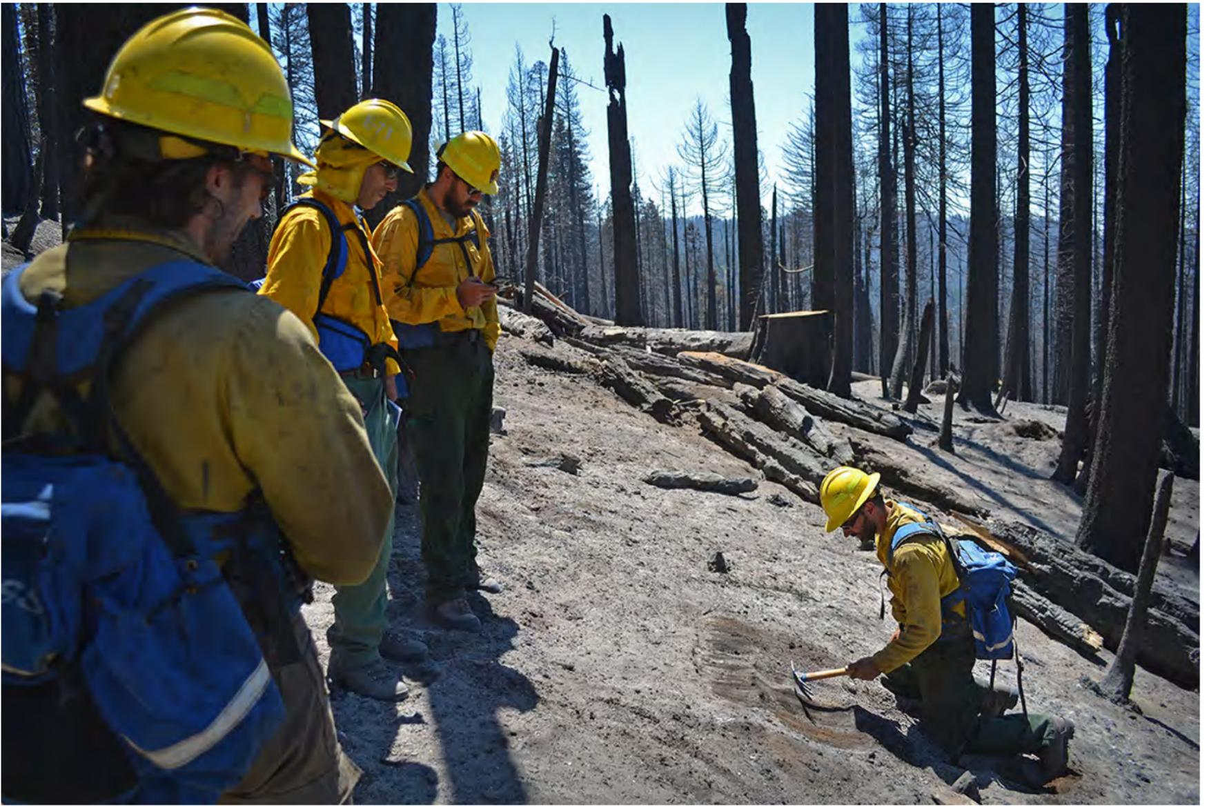
Samuel Prentice measures soil hydrophobicity in a high-severity burn area on the Ferguson Fire with his colleagues on the BAER team. After creating different depths in the soil, he pours droplets of water onto each depth to determine the extent of how much water soaks into it (hydrophilic) or rolls off of it (hydrophobic). This ultimately tells resource advisors on the BAER team which types of soil erosion control measures need to be taken for the area (USFS).
